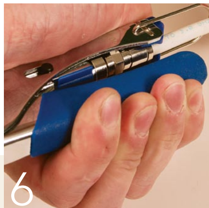
6 Squeeze the crimper firmly to compress the fitting onto the end of the cable.
