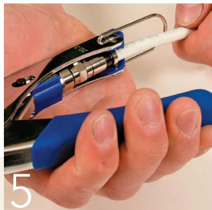
5 Open the crimper tool, and insert the cable assembly into the handle.
