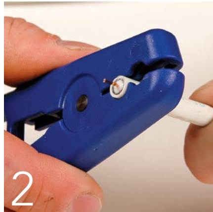
2 Carefully strip away ¼ in. of the outer jacket to expose the braided shielding.
