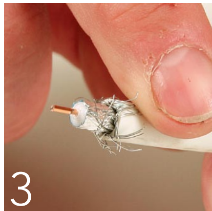
3 Gently fold back the braided shielding to expose the foil-covered white dielectric.
