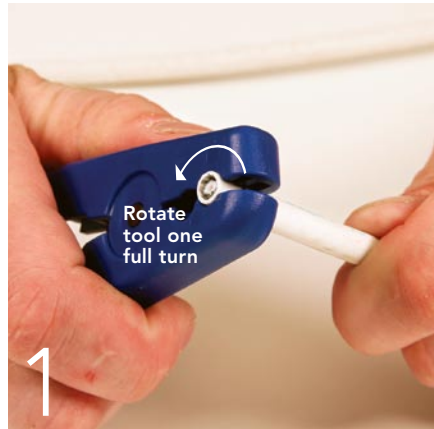
1 Remove ¼ in. of the outer layers to expose the central copper conductor.
