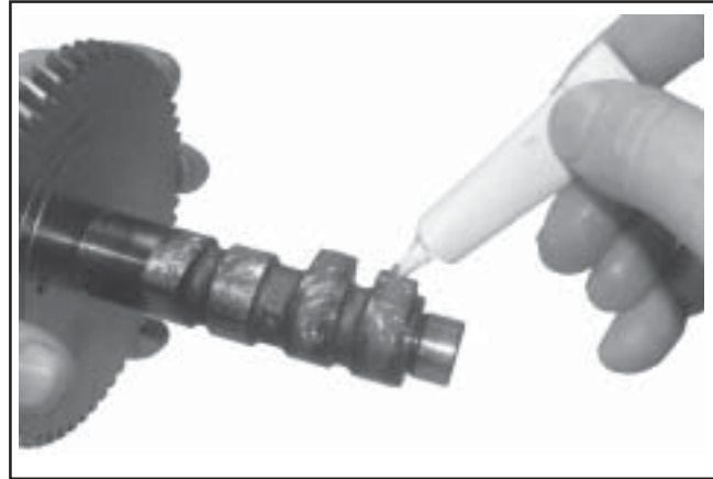
Figure 11-12. Apply Camshaft Lubricant to Cam Lobes.
