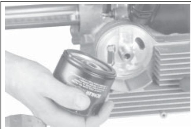
Figure 11-101. Installing New Oil Filter.
