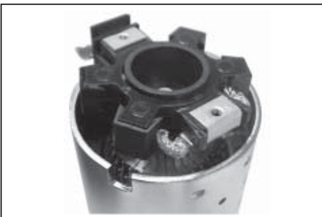
Figure 8-67. Installing Brush Holder Assembly with Supplied Tube.
