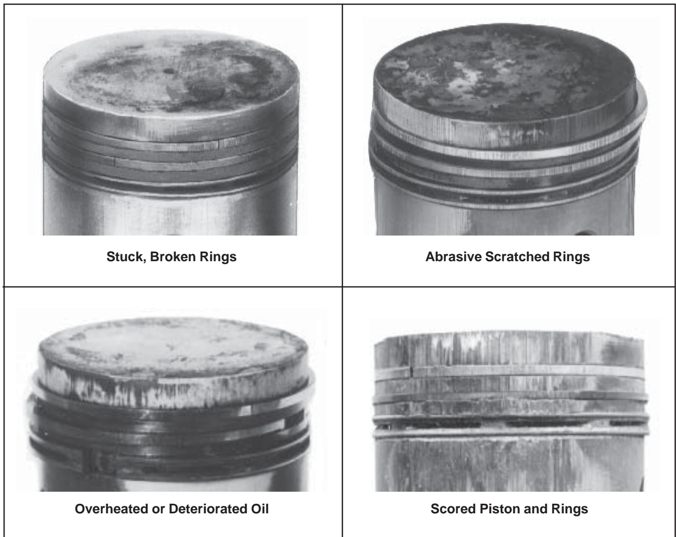
Figure 10-8. Common Types of Piston Damage.
