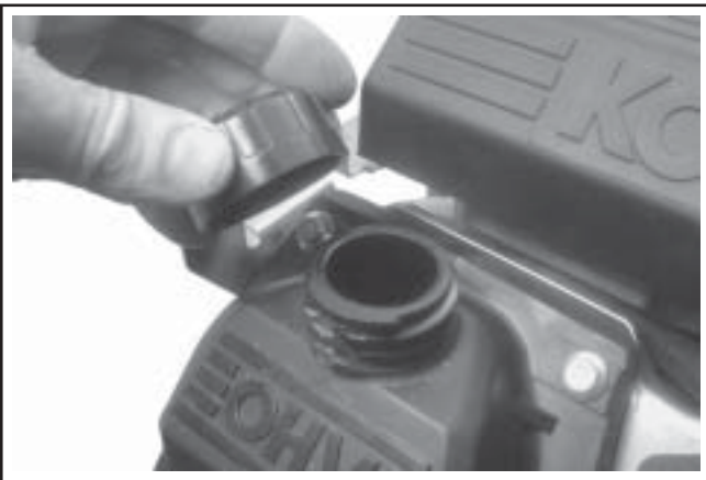
Figure 11-105. Reinstalling Oil Fill Cap (Some Models).
