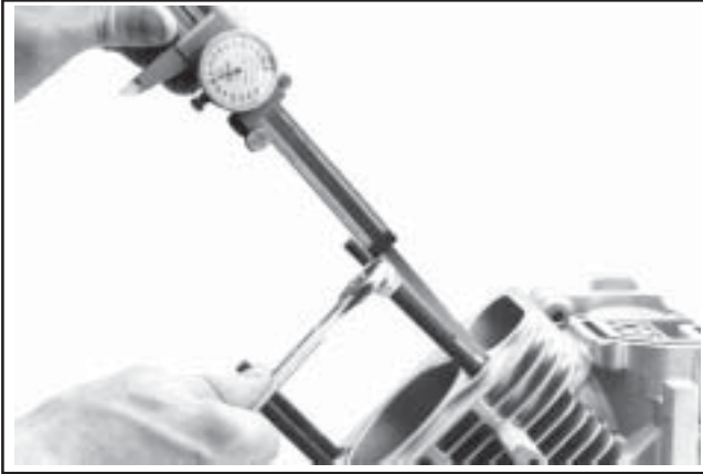
Figure 11-43. Installing New Mounting Studs to Specified Height.
