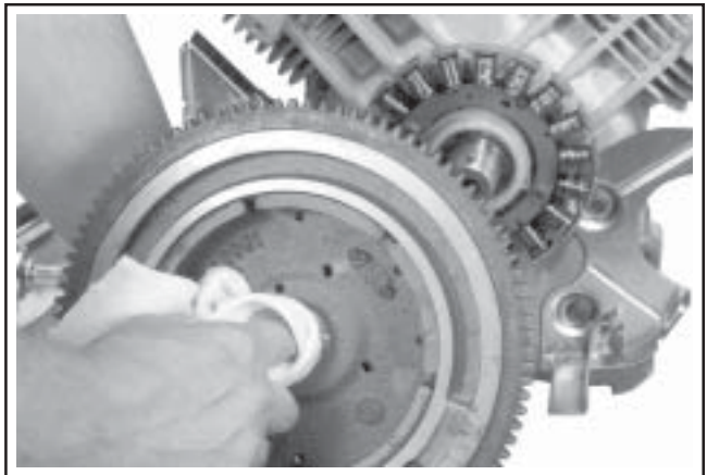
Figure 11-27. Clean and Dry Flywheel Hub.
