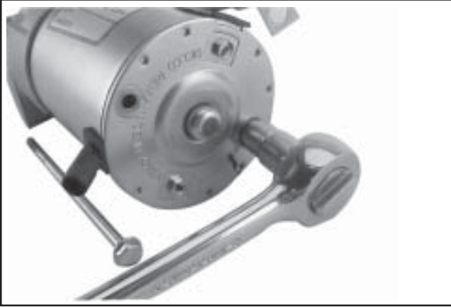
Figure 8-48. Removing Thru Bolts.
