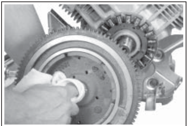
Figure 11-27. Clean and Dry Flywheel Hub.
