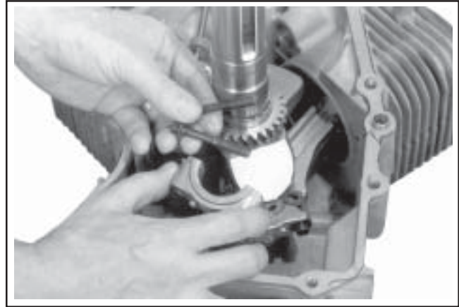
Figure 9-71. Mark End Cap with Cylinder Number Before Removal.
