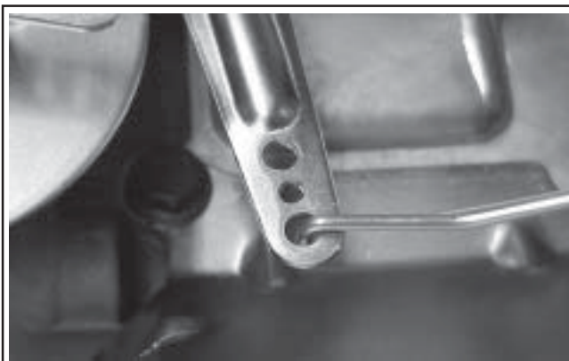
Figure 5B-40. Throttle Link in Center of Hole.
