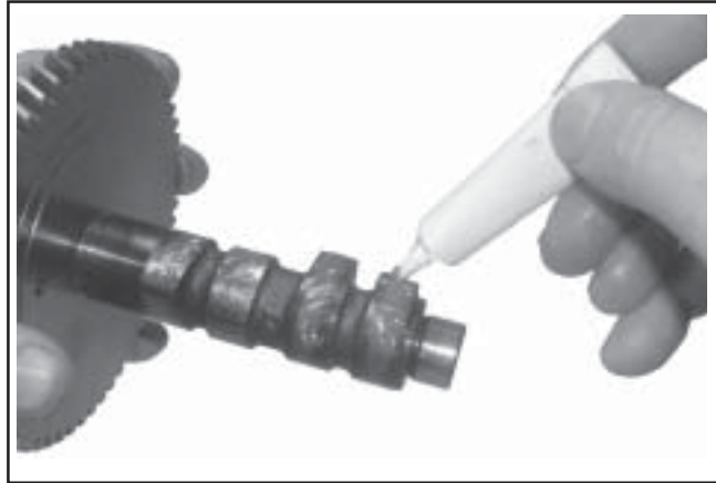
Figure 11-12. Apply Camshaft Lubricant to Cam Lobes.
