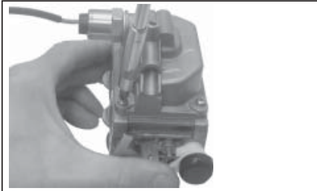
Figure 5-21. Installing Fuel Bowl.
