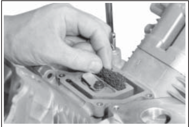
Figure 11-57. Installing New Breather Filter.
