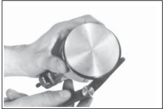
Figure 10-10. Measuring Piston Ring Side Clearance.
