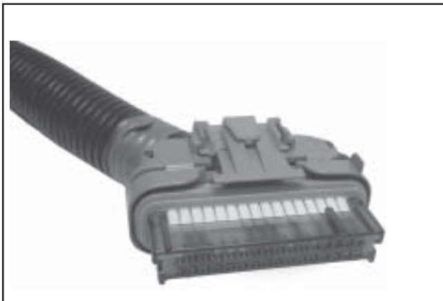
Figure 5B-25. “32 Pin” (MSE 1.1) Plastic-Cased ECU Connector.
