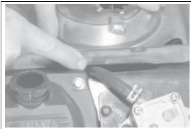
Figure 11-93. Fuel Inlet Line Detail.
