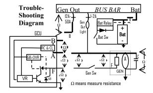
No voltage regulation or Generator not Coming on-line With the Bat & Field switches on, engine off,
