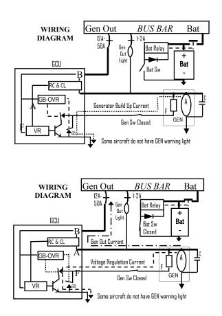
**Caution:** Check the condition of the battery. A depleted /discharged battery will draw excessive current and could trigger the Current Limiter function to turn off the GCU's voltage regulator.
