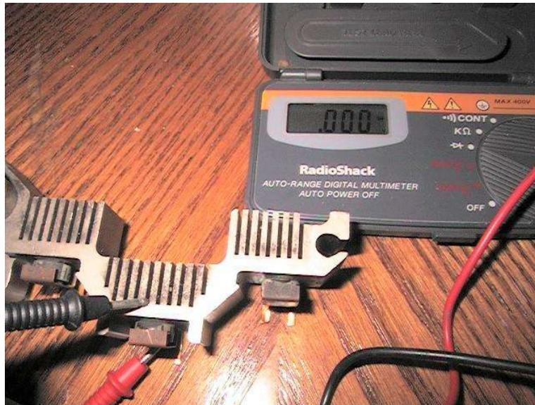
I hooked up three 10-gauge wires to the stator leads leading the 3 phase outside the case to the external rectifier. This is what the external rectifier looks like with the 3 phase wires going to it mounted on the alternator support bracket:
