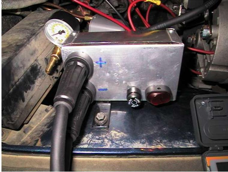
This is the simple control box. It ended up being too small with the relay and the thick cables running inside. It contains a 30A automotive relay, a 10A fuse holder, a lighted 30A rocker switch and two female welding lead quick connect sockets. I will probably upgrade to a larger box that will accommodate a panel voltmeter and a 110V outlet.
