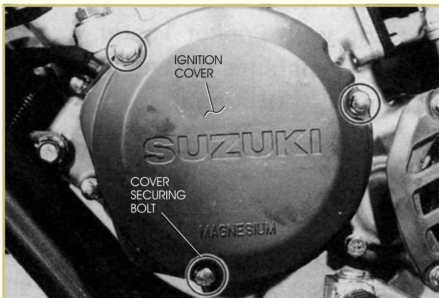
FIGURE 21 —The ignition system cover will normally be found on the left side of the motorcycle or ATV engine. (Courtesy of American Suzuki Motor Corporation)
